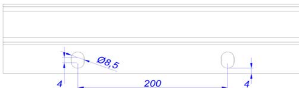
Foratura standard per C-14 e C-15 Standard drilling for C-14 and C-15
